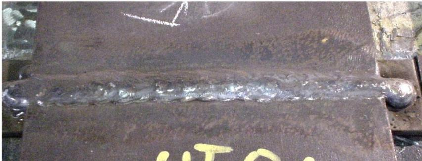
Figure 1 – MCAW butt weld (with backing) with excessive weld height
