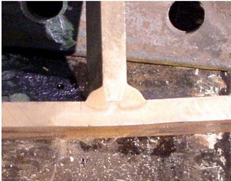
Figure 2 – Photo of macro etch for MCAW weld.
