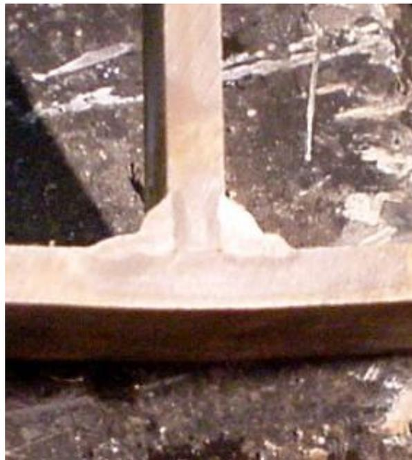
Figure 3 – Photo of macro etch for SMAW weld.
