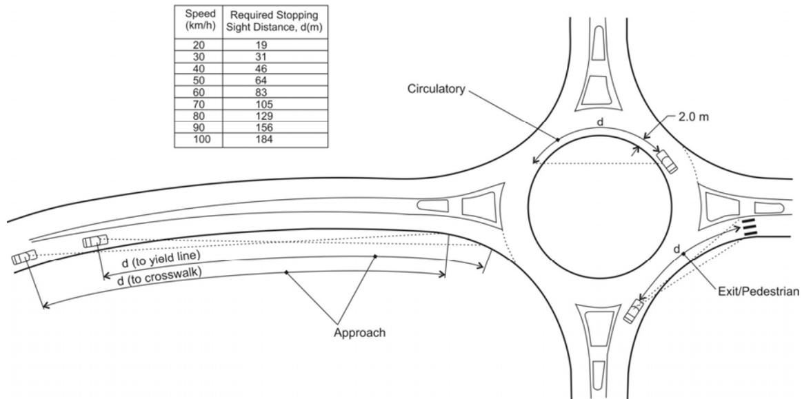
Figure 2.1: Critical Stopping Sight Distance
