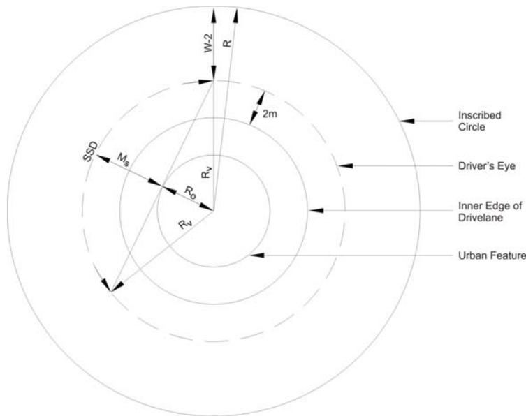
Figure 3.2: Roundabout Dimensions
