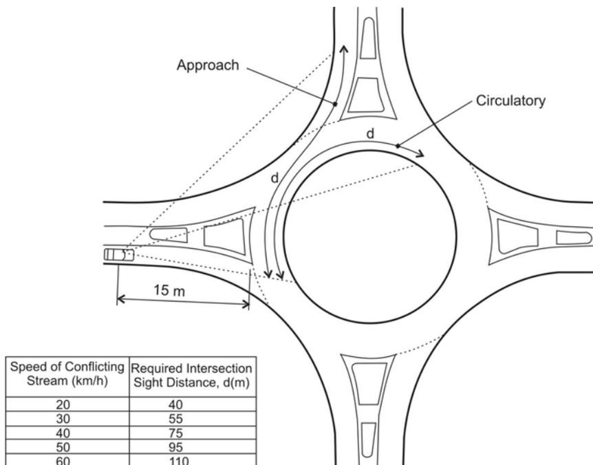
Figure 2.2: Intersection Sight Distance Requirements at Roundabouts
