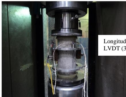
a) Compression Test Set-up
